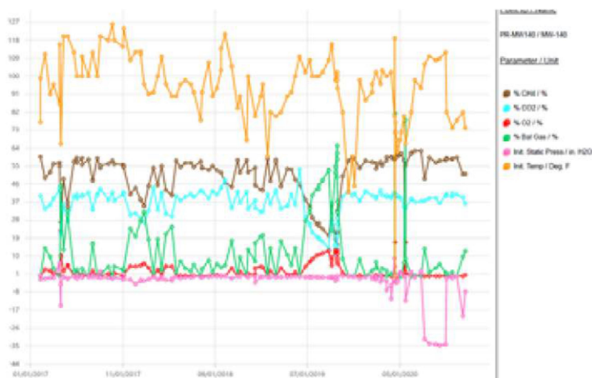
Figure 3 - Graphical depiction of oxidation phase in well data.
